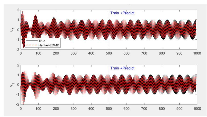
The eDMD model is trained on 500 seconds of the dimer dynamics, and then predicts the future of the system up until 1000 seconds. The red curve indicates the eDMD trajectory, and the black curve is the true dynamics.
